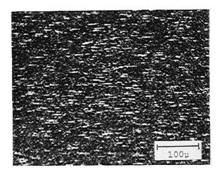
Fig. 5  $\label{eq:S-Ka} \text{S-K}_{\alpha} \text{ radiation profile of the }$  same surface.
